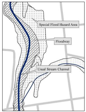
that must be reserved in order to discharge the base flood without cumulatively increasing the water surface elevation more than one foot at any point.
