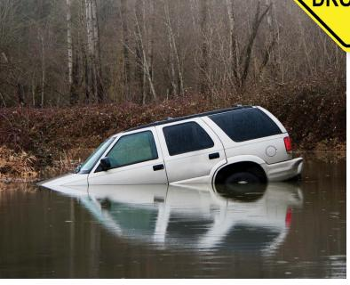
**Forces on Vehicles Crossing Streams** The car will be carried when: Buoyancy force Greater Than Vehicle Weight **Friction Force** Buoyancy Force There is no friction force once the vehicle is lifted off the road Nearly half of all flood fatalities are vehicle related
