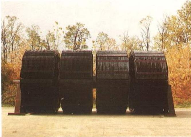
The Walker Process Rotating Biological Contactor provides a simple and effective method of providing secondary and/or advanced wastewater treatment by a natural biological process.
